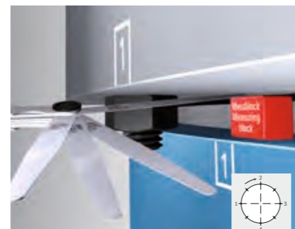
Figure 37: Basic setup for measuring the axial reduction with a feeler gauge
