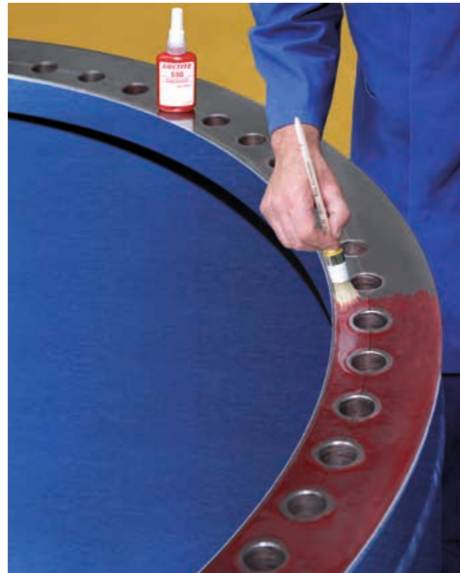
Figure 16: Application of Loctite
