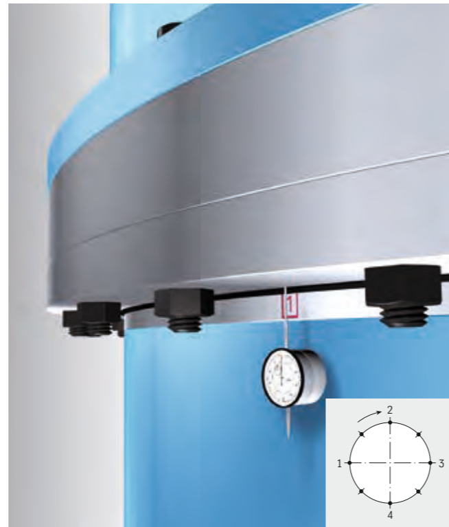
Figure 34: Basic setup for measuring the tilting clearance
