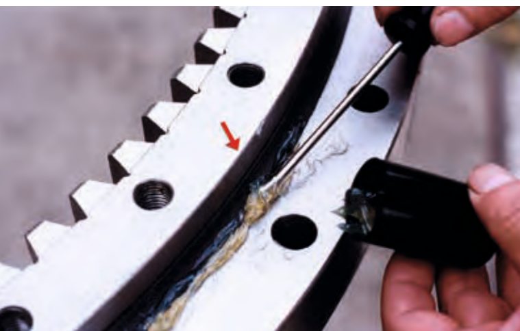
Figure 45: Taking a sample of grease from the sealing lip
